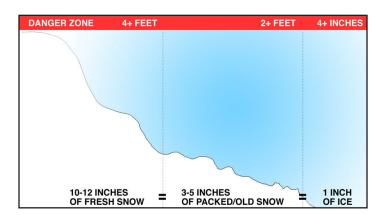
Not all types of snow weigh the same. The above chart looks at the differences between fresh snow, packed snow, and ice. A structural engineer can determine the maximum loads your roof can withstand, as well as provide practical solutions to improve roof strength.
